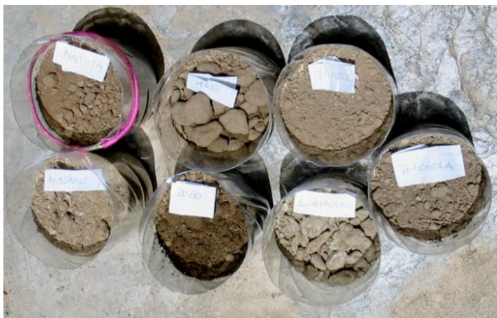
Illustration 5: Soil samples from the check dam fields; each container is filled up with 0.5 litre of soil; Alitena, August 2003
